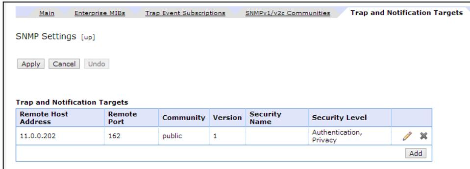
Figure 3-16. Configure SNMP Settings – Trap and Notification Targets Tab
